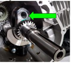
Figure 5 – Flywheel must have Loncin original marking 168F manufacturers marking
