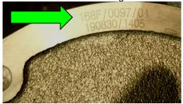
Figure 7 – Camshaft must have Loncin original marking containing the LC168F number.
