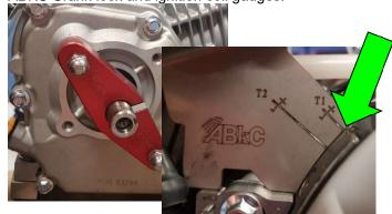
Notes for Figure 8 – Ignition timing advancement will be checked using the ABKC crank lock as shown in the left image. When a feeler gauge is placed in the T1 slot on the coil gauge, it **must not** land on the magnet area – if it **does** then it will be considered too far advanced and therefore illegal. The right image shows an example of the maximum ignition position with the slot just at the front edge of the magnet area.
