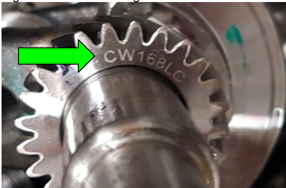
Figure 4 – Crank Timing Collar must have Loncin original marking CW168LC and not be rotated on the crank.
