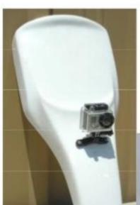
The mounting location is on the front panel. The installation kit must be fixed horizontally, in the middle of the panel, and between 300 mm (11.810") and 400 mm (15.748") from the upper edge.
